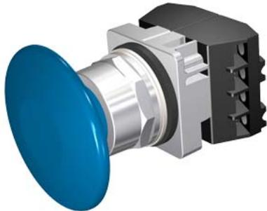
30mm Command/52, Chrome Finish Heavy Duty, Watertight/Oiltight Complete Metal Unit Push-Pull Operator Non-Illuminated Mushroom Head Cap Large 2 1/2" (63.5 mm) Plastic, Blue 2 Position Maintained, Pull-to-Release with 2 N.O. - 2 N.C. Heavy Duty Contacts, A600/P600 UL Listed, CSA Certified NEMA 1,3,3R,4,4X,12,13 & Automotive Standards
