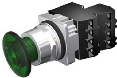
30mm Command/52, Chrome Finish Heavy Duty, Watertight/Oiltight Complete Metal Unit Illuminated Push-Pull Operator Full Voltage, 6V AC/DC Incandescent Lamp Mushroom Head Cap Small 1 3/4" (44.5 mm) Plastic, Green 3 Position Pull-Momentary/Push-Maintained 1 N.C.+1 N.C. Extra Late Break Heavy Duty Contacts, A600/P600 UL Listed, CSA Certified NEMA 1,3,3R,4,4X,12,13 & Automotive Standards
