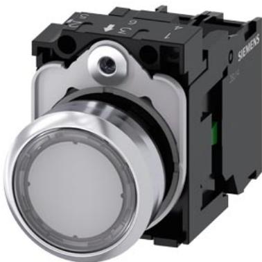
Illuminated pushbutton, 22 mm, round, metal, shiny, clear, pushbutton, flat, momentary contact type, with holder, 1NO, LED module with integrated LED 24 V AC/DC, screw terminal, with laser labeling, upper case and lower case, always upper case at beginning of line
