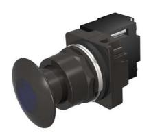
30mm BlackMax, Epoxy Coated Corrosion Resistant Complete Metal Unit Illuminated Push-Pull Operator Full Voltage, 120V AC/DC Incandescent Lamp Mushroom Head Cap Small 1 3/4" (44.5 mm) Metal, Black with Blue Lens 3 Position Momentary UL Listed, CSA Certified NEMA 1,3,3R,4,4X,12,13 & Automotive Standards
