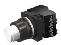
30mm BlackMax, Epoxy Coated Corrosion Resistant Complete Metal Unit PTT / Illuminated Pushbutton Transformer type, 480V AC LED Lamp Extended Button Plastic Lens, White 2 Position Momentary with 1 N.O. - 1 N.C. Heavy Duty Contacts, A600/P600 UL Listed, CSA Certified NEMA 1,3,3R,4,4X,12,13 & Automotive Standards
