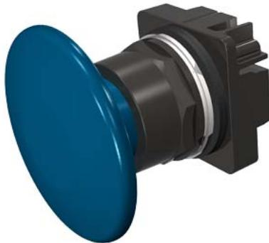
30mm BlackMax, Epoxy Coated Corrosion Resistant Metal Operator, Round Push-Pull Operator Non-Illuminated Mushroom Head Cap Large 2 1/2" (63.5 mm)
