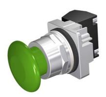
30mm Command/52, Chrome Finish Heavy Duty, Watertight/Oiltight Complete Metal Unit Push-Pull Operator Non-Illuminated Mushroom Head Cap Small 1 3/4" (44.5 mm) Plastic, Green 2 Position Maintained, Pull-to-Release with 1 N.O. - 1 N.C. Heavy Duty Contacts, A600/P600 UL Listed, CSA Certified NEMA 1,3,3R,4,4X,12,13 & Automotive Standards
