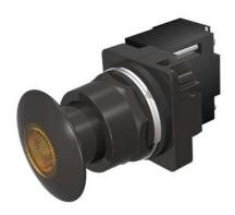
30mm BlackMax, Epoxy Coated Corrosion Resistant Complete Metal Unit Illuminated Push-Pull Operator Full Voltage, 6V AC LED Lamp Mushroom Head Cap Small 1 3/4" (44.5 mm) Metal, Black with Amber Lens 3 Position Pull-Momentary/Push-Maintained UL Listed, CSA Certified NEMA 1,3,3R,4,4X,12,13 & Automotive Standards
