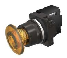
30mm BlackMax, Epoxy Coated Corrosion Resistant Complete Metal Unit Illuminated Push-Pull Operator Transformer type, 240V AC Incandescent Lamp Mushroom Head Cap Small 1 3/4" (44.5 mm) Plastic, Amber 2 Position Maintained, Pull-to-Release UL Listed, CSA Certified NEMA 1,3,3R,4,4X,12,13 & Automotive Standards
