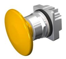
30mm Command/52, Chrome Finish Heavy Duty, Watertight/Oiltight Metal Operator, Round Push-Pull Operator Non-Illuminated Mushroom Head Cap Large 2 1/2" (63.5 mm) Plastic, Yellow 2 Position Maintained, Pull-to-Release UL Listed, CSA Certified NEMA 1,3,3R,4,4X,12,13 & Automotive Standards
