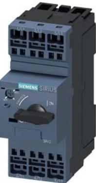
Circuit breaker size S0 for motor protection, CLASS 10 A-release 11...16 A N-release 208 A Spring-type terminal switching capacity 30 kA at 600 V according to UL/CSA
