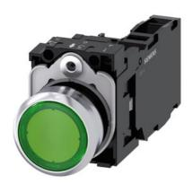
Illuminated pushbutton, 22 mm, round, metal, shiny, green, pushbutton, flat, momentary contact type, with holder, 1 NO+1 NC, LED module with integrated LED 24 V AC/DC, screw terminal, with laser labeling, inscription or symbol Customer-specific selection with SIRIUS ACT configurator (CIN)
