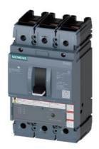
circuit breaker 3VA5 UL frame 250 3-pole, starter protection TM120M, AM, In=200A without overload protection short-circuit protection li=6...12 x In nut keeper kit on both sides
