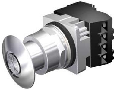
30mm Command/52, Chrome Finish Heavy Duty, Watertight/Oiltight Complete Metal Unit Illuminated Push-Pull Operator Transformer type, 120V AC Incandescent Lamp Mushroom Head Cap Small 1 3/4" (44.5 mm) Metal, Chrome with Clear Lens 2 Position Maintained, Pull-to-Release with 1 N.O. - 1 N.C. Heavy Duty Contacts, A600/P600 UL Listed, CSA Certified NEMA 1,3,3R,4,4X,12,13 & Automotive Standards
