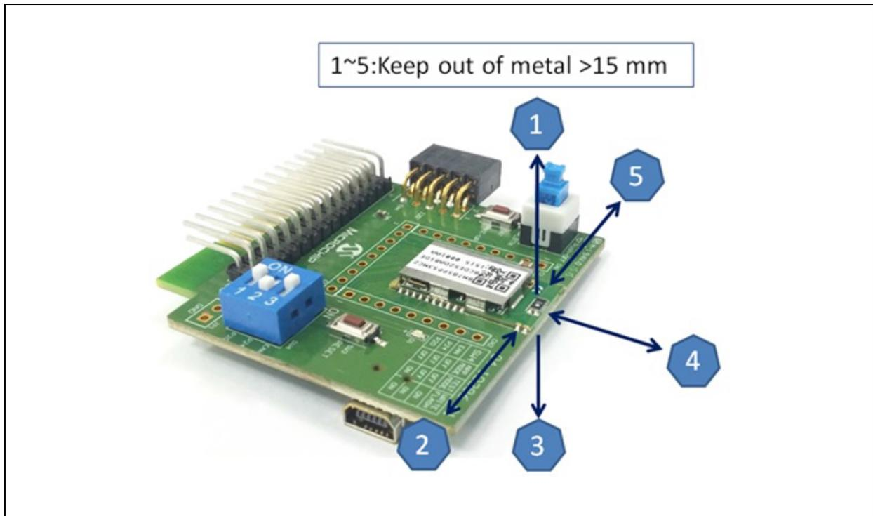
**Note:** For additional information on free space for antenna placement design, refer to the design rule document of the antenna manufacturer.
