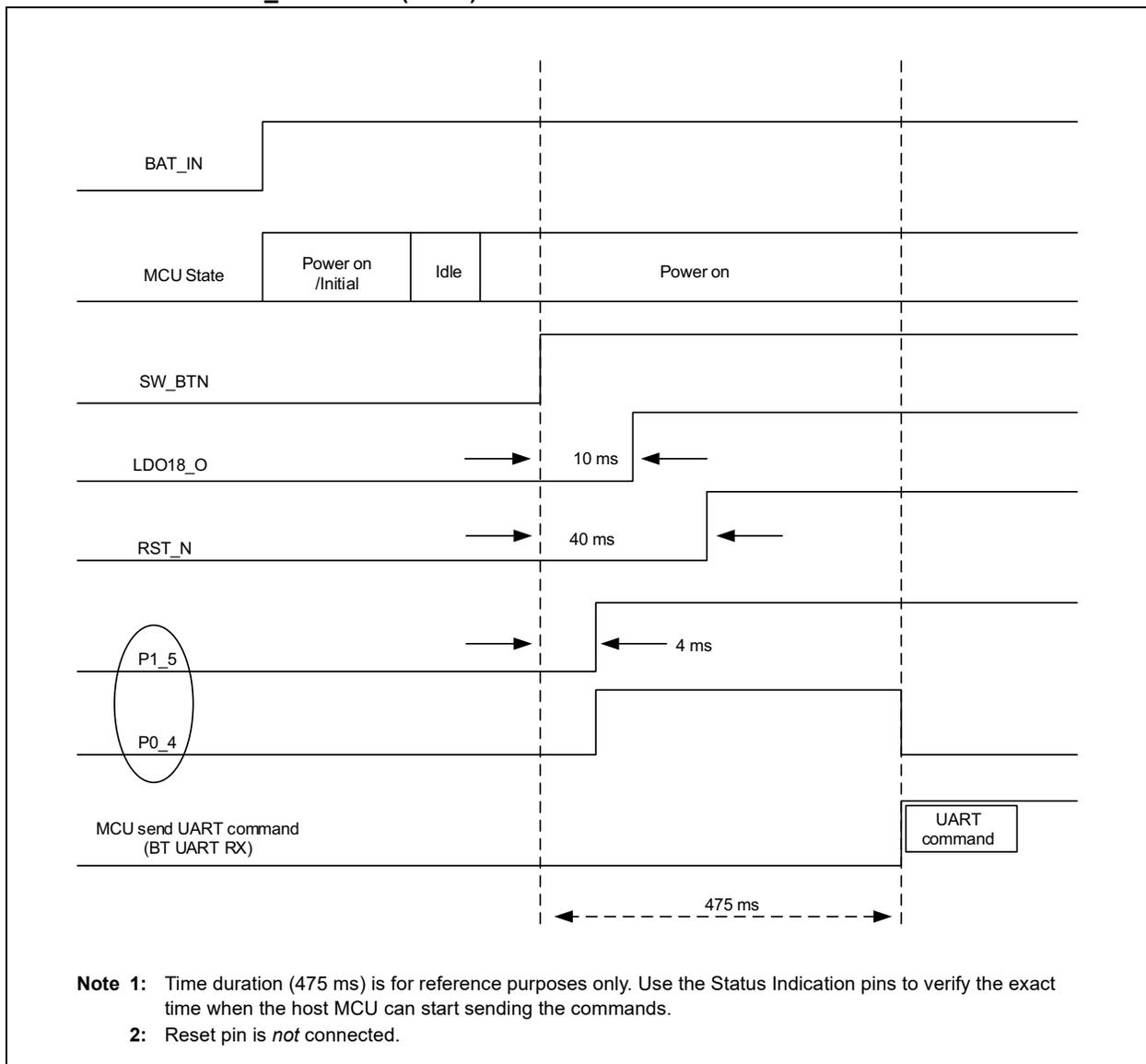
**FIGURE 2-3: SW\_BTN TIME (LOW) AT ACCESS STATES<sup>(1)</sup>**
