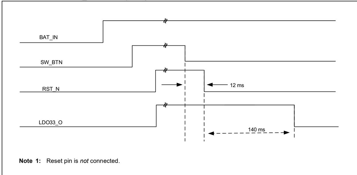
**FIGURE 2-4: SW\_BTN TIME (LOW) AT LINK STATES<sup>(1,2)</sup>**
