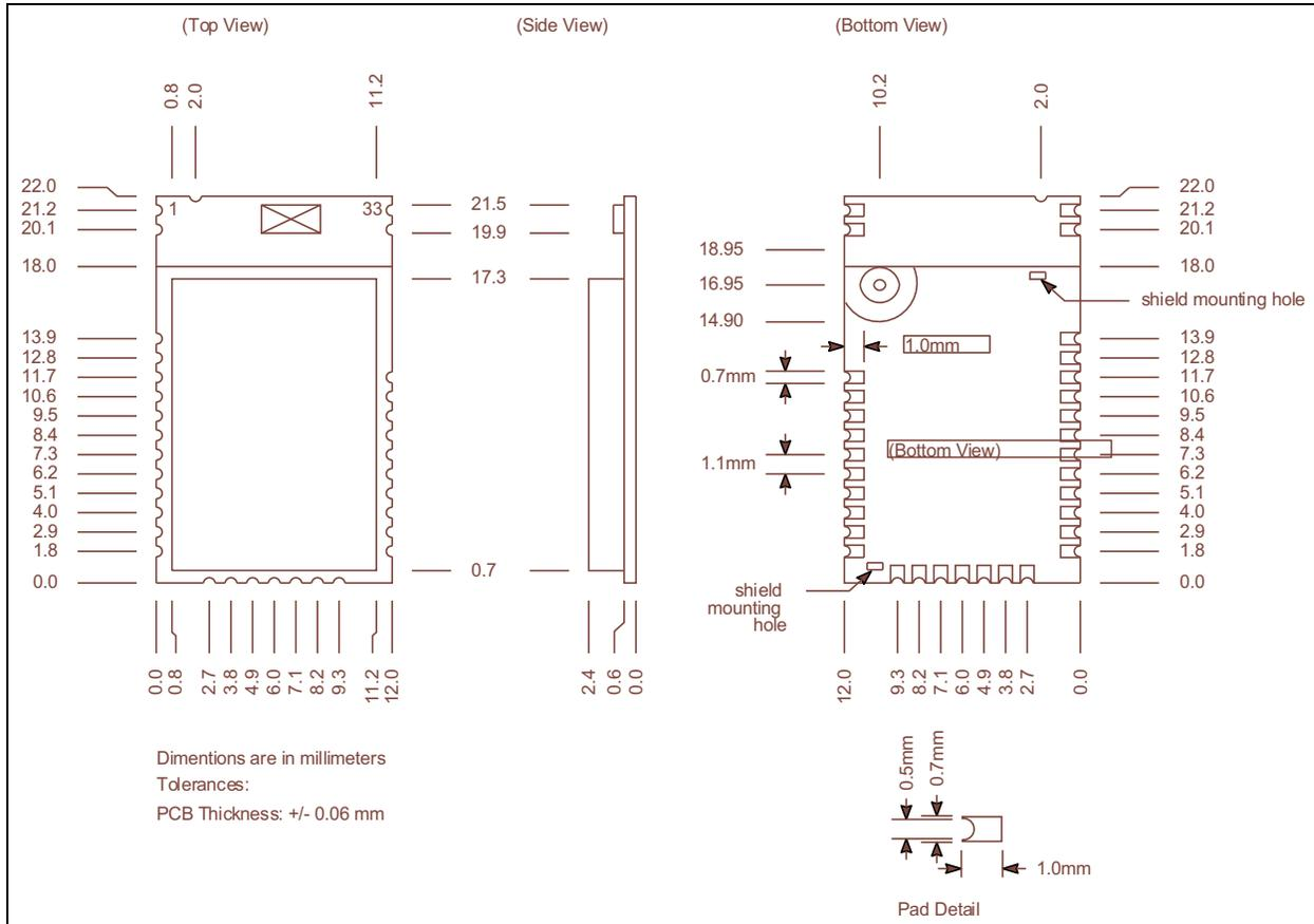
Figure 5-2 illustrates the recommended host PCB footprint.
