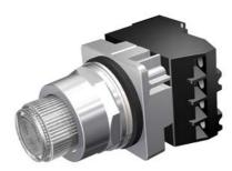
30mm Command/52, Chrome Finish Heavy Duty, Watertight/Oiltight Complete Metal Unit PTT / Illuminated Pushbutton Full Voltage, 120V AC/DC Incandescent Lamp Extended Button Plastic Lens, Clear 2 Position Momentary with 1 N.O. - 1 N.C. Heavy Duty Contacts, A600/P600 UL Listed, CSA Certified NEMA 1,3,3R,4,4X,12,13 & Automotive Standards
