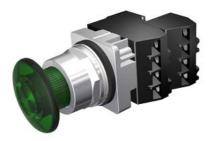
30mm Command/52, Chrome Finish Heavy Duty, Watertight/Oiltight Complete Metal Unit Illuminated Push-Pull Operator Transformer type, 480V AC Incandescent Lamp Mushroom Head Cap Small 1 3/4" (44.5 mm) Plastic, Green 3 Position Pull-Momentary/Push-Maintained 1 N.C.+1 N.C. Extra Late Break Heavy Duty Contacts, A600/P600 UL Listed, CSA Certified NEMA 1,3,3R,4,4X,12,13 & Automotive Standards
