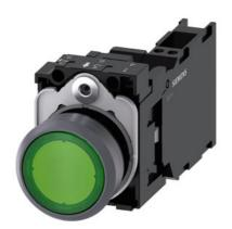
Illuminated pushbutton, 22 mm, round, plastic with metal front ring, green, pushbutton, flat, momentary contact type, with holder, 1 NO+1 NC, LED module with integrated LED 24 V AC/DC, spring-type terminal, with laser labeling, upper case
