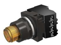
30mm BlackMax, Epoxy Coated Corrosion Resistant Complete Metal Unit PTT / Illuminated Pushbutton Full Voltage, 12V AC/DC Incandescent Lamp Extended Button Plastic Lens, Amber 2 Position Momentary with 1 N.O. - 1 N.C. Heavy Duty Contacts, A600/P600 UL Listed, CSA Certified NEMA 1,3,3R,4,4X,12,13 & Automotive Standards
