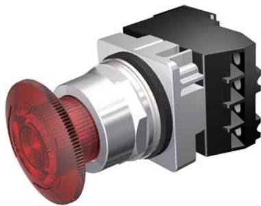
30mm Command/52, Chrome Finish Heavy Duty, Watertight/Oiltight Complete Metal Unit Illuminated Twist-to-Release Full Voltage, 120V AC/DC Incandescent Lamp Mushroom Head Cap Small 1.79" (45 mm) Plastic Cap, Red 2 Position Maintained, Twist-to-Release with 1 N.O. - 1 N.C. Heavy Duty Contacts, A600/P600 UL Listed, CSA Certified NEMA 1,3,3R,4,4X,12,13 & Automotive Standards
