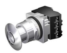
30mm Command/52, Chrome Finish Heavy Duty, Watertight/Oiltight Complete Metal Unit Illuminated Push-Pull Operator Transformer type, 480V AC Incandescent Lamp Mushroom Head Cap Small 1 3/4" (44.5 mm) Metal, Chrome with Clear Lens 2 Position Maintained, Pull-to-Release with 1 N.O. - 1 N.C. Heavy Duty Contacts, A600/P600 UL Listed, CSA Certified NEMA 1,3,3R,4,4X,12,13 & Automotive Standards
