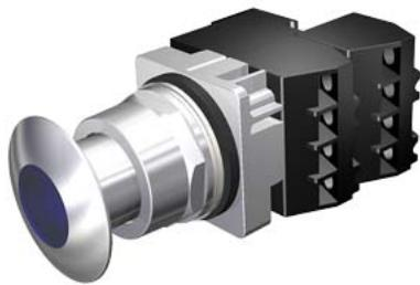
30mm Command/52, Chrome Finish Heavy Duty, Watertight/Oiltight Complete Metal Unit Illuminated Push-Pull Operator Full Voltage, 6V AC LED Lamp Mushroom Head Cap Small 1 3/4" (44.5 mm) Metal, Chrome with Blue Lens 3 Position Pull-Momentary/Push-Maintained 1 N.C.+1 N.C. Extra Late Break Heavy Duty Contacts, A600/P600 UL Listed, CSA Certified NEMA 1,3,3R,4,4X,12,13 & Automotive Standards
