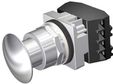
30mm Command/52, Chrome Finish Heavy Duty, Watertight/Oiltight Complete Metal Unit Push-Pull Operator Non-Illuminated Mushroom Head Cap Small 1.73" (44 mm) Metal, Chrome 3 Position Pull-Momentary/Push-Maintained 1 N.C.+1 N.C. Extra Late Break Heavy Duty Contacts, A600/P600 UL Listed, CSA Certified NEMA 1,3,3R,4,4X,12,13 & Automotive Standards
