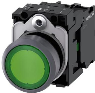
Illuminated pushbutton, 22 mm, round, plastic with metal front ring, green, pushbutton, flat, momentary contact type, with holder, 1NO, LED module with integrated LED 230 V AC, screw terminal, with laser labeling, upper case and lower case, Always upper case at the beginning of the word
