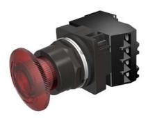
30mm BlackMax, Epoxy Coated Corrosion Resistant Complete Metal Unit Illuminated Twist-to-Release Full Voltage, 120V AC/DC Incandescent Lamp Mushroom Head Cap Small 1.79" (45 mm) Plastic Cap, Red 2 Position Maintained, Twist-to-Release with 1 N.O. - 1 N.C. Heavy Duty Contacts, A600/P600 UL Listed, CSA Certified NEMA 1,3,3R,4,4X,12,13 & Automotive Standards
