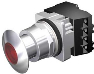
30mm Command/52, Chrome Finish Heavy Duty, Watertight/Oiltight Complete Metal Unit Illuminated Push-Pull Operator Transformer type, 480V AC LED Lamp Mushroom Head Cap Small 1 3/4" (44.5 mm) Metal, Chrome with Red Lens 2 Position Maintained, Pull-to-Release with 1 N.O. - 1 N.C. Heavy Duty Contacts, A600/P600 UL Listed, CSA Certified NEMA 1,3,3R,4,4X,12,13 & Automotive Standards
