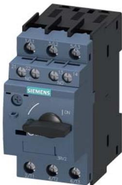
Circuit breaker size S0 for motor protection, CLASS 10 A-release 0.7...1 A N-release 13 A screw terminal Standard switching capacity with transverse auxiliary switches 1 NO+1 NC
