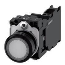
Illuminated pushbutton, 22 mm, round, plastic, clear, pushbutton, flat, momentary contact type, with holder, 1 NO+1 NC, LED module with integrated LED 24 V AC/DC, spring-type terminal, with laser labeling, upper case and lower case, Always upper case at the beginning of the word
