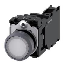
Illuminated pushbutton, 22 mm, round, plastic with metal front ring, white, pushbutton, flat, momentary contact type, with holder, 1 NO+1 NC, LED module with integrated LED 24 V AC/DC, spring-type terminal, with laser labeling, inscription or symbol Customer-specific selection with SIRIUS ACT configurator (CIN)
