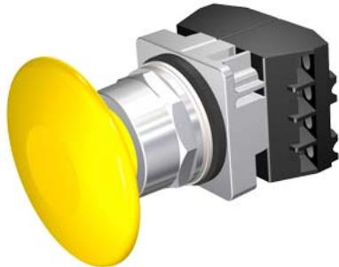
30mm Command/52, Chrome Finish Heavy Duty, Watertight/Oiltight Complete Metal Unit Push-Pull Operator Non-Illuminated Mushroom Head Cap Large 2 1/2" (63.5 mm) Plastic, Yellow 3 Position Momentary 1 N.C.+1 N.C. Extra Late Break Heavy Duty Contacts, A600/P600 UL Listed, CSA Certified NEMA 1,3,3R,4,4X,12,13 & Automotive Standards
