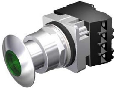
30mm Command/52, Chrome Finish Heavy Duty, Watertight/Oiltight Complete Metal Unit Illuminated Push-Pull Operator Transformer type, 480V AC LED Lamp Mushroom Head Cap Small 1 3/4" (44.5 mm) Metal, Chrome with Green Lens 2 Position Maintained, Pull-to-Release with 1 N.O. - 1 N.C. Heavy Duty Contacts, A600/P600 UL Listed, CSA Certified NEMA 1,3,3R,4,4X,12,13 & Automotive Standards
