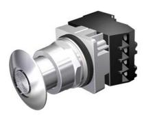
30mm Command/52, Chrome Finish Heavy Duty,Watertight/Oiltight Complete Metal Unit Illuminated Push-Pull Operator Transformer type, 480V AC LED Lamp Mushroom Head Cap Small 1 3/4" (44.5 mm) Metal, Chrome with Clear Lens 2 Position Maintained, Pull-to-Release with 1 N.O. - 1 N.C. Heavy Duty Contacts, A600/P600 UL Listed, CSA Certified NEMA 1,3,3R,4,4X,12,13 & Automotive Standards
