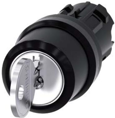
RONIS key-operated switch, 22 mm, round, plastic, lock number 455, with 2 keys, 3 switch positions I-O-II, latching, actuating angle 2x45°, 10:30h/12h/13:30h, Key removal I+O+II, with laser labeling, upper case
