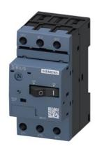
Circuit breaker size S00 for motor protection, CLASS 10 A-release 12...16 A N-release 208 A Screw terminal Standard switching capacity Special version with limited ON period Use only on request
