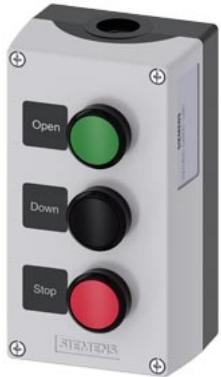
enclosure for command devices, 22 mm, round, enclosure material plastic, enclosure top part gray, 3 control points plastic, C=Pushbutton green, label: Open, 1 NO, 1 NC, screw terminal, B=Pushbutton black, label: Close, 1 NO, 1 NC, screw terminal, A=Pushbutton red, label: Stop, 1 NO, 1 NC, screw terminal, floor mounting, 1xM20 each on top and bottom, Labels glued in
