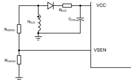
Fig. voltage detection and feedback
