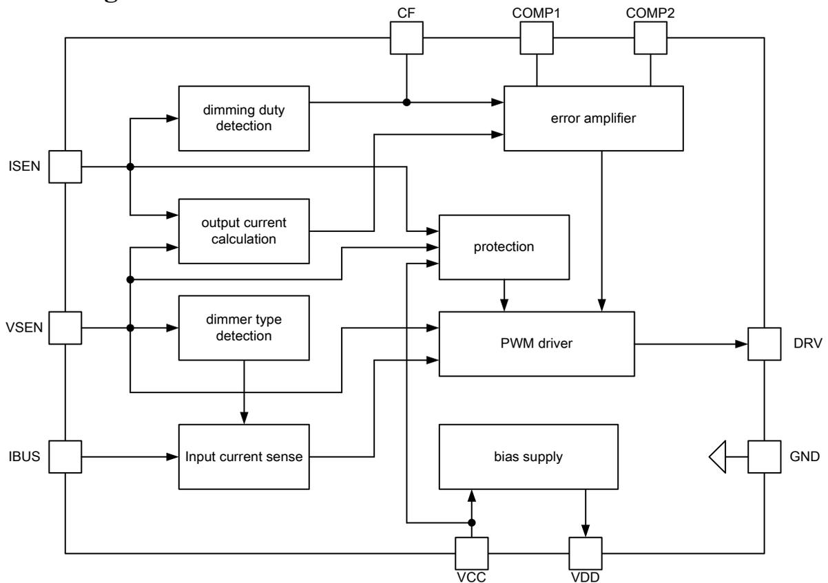
Figure3. Block Diagram
