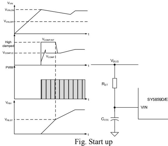
This operation is aimed to build up enough output voltage for auxiliary winding bias supply as quickly as possible. It is enabled only one time just when  $V_{VIN}$  is over  $V_{VIN,ON}$ .
