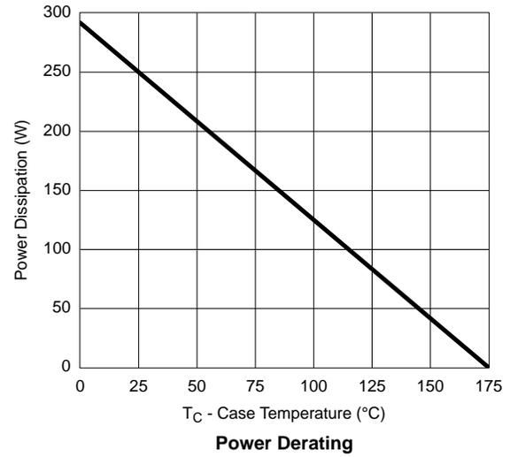
\*The power dissipation P<sub>D</sub> is based on T<sub>J(max)</sub> = 175 °C, using junction-to-case thermal resistance, and is more useful in settling the upper dissipation limit for cases where additional heatsinking is used. It is used to determine the current rating, when this rating falls below the package limit.
