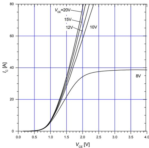
**Figure 7. Typical output characteristics**
