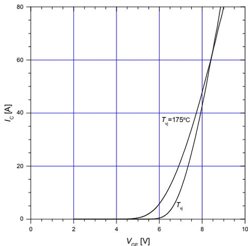
**Figure 9. Gate threshold voltage**
