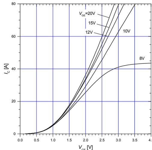
**Figure 8. Typical transfer characteristics**
