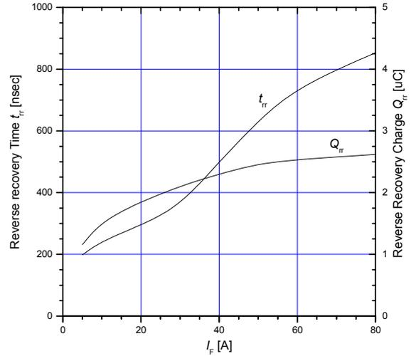
Figure 18. Typical reverse recovery loss vs.  $I_F$
