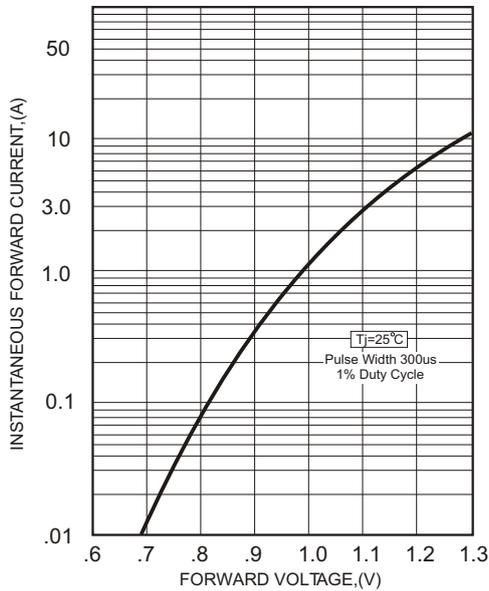
FIG.2-TYPICAL FORWARD CURRENT DERATING CURVE
