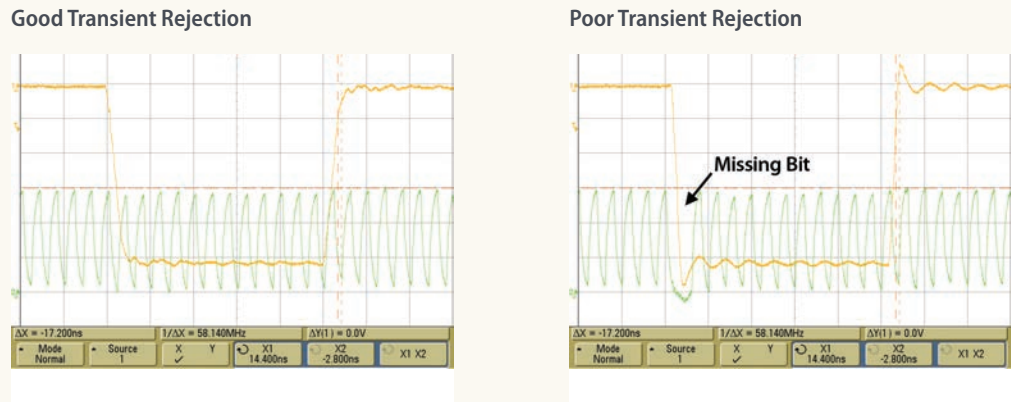
Figure 6. Missing Bit due to Poor Transient Immunity.
