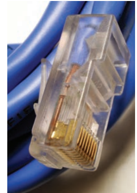
Figure 4. CAT5 cables with RJ45 connectors.
