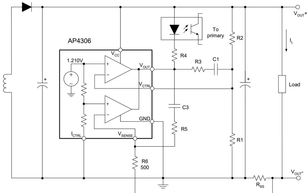
$$V_{OUT} = V_{REF} \times \frac{R1 + R2}{R1} - (I_L \times R_{SS})$$
