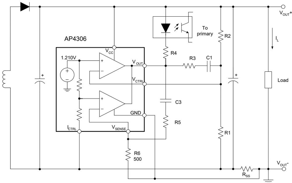
$$V_{OUT} = [V_{REF} + (I_L \times R_{SS})] \times \frac{R1 + R2}{R1} - (I_L \times R_{SS})$$
