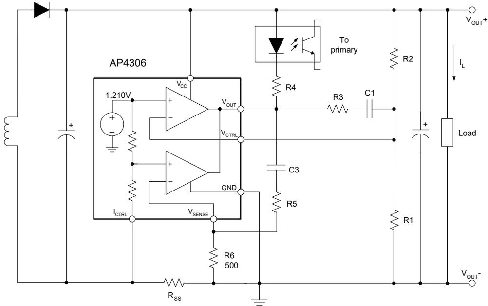
$$V_{OUT} = V_{REF} \times \frac{R1 + R2}{R1}$$
