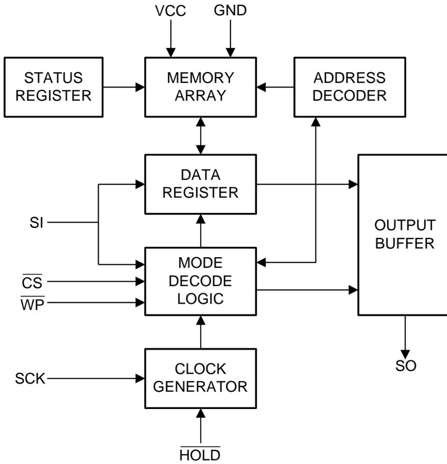
Figure 2: Block Diagram
