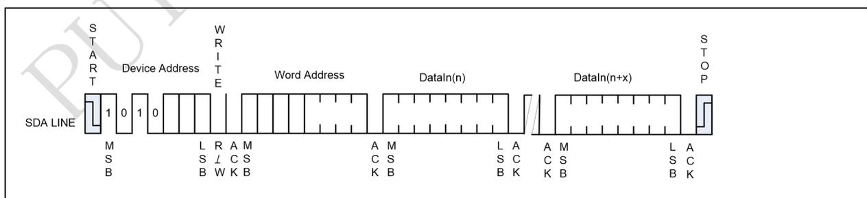
The lower four bits of the data word address are internally incremented following the receipt of each data word. The higher data word address bits are not incremented, retaining the memory page row location. When the word address, internally generated, reaches the page boundary, the following byte is placed at the beginning of the same page. If more than 16 data words are transmitted to the P24C02C/P24C04C/P24C08C/P24C16C,
