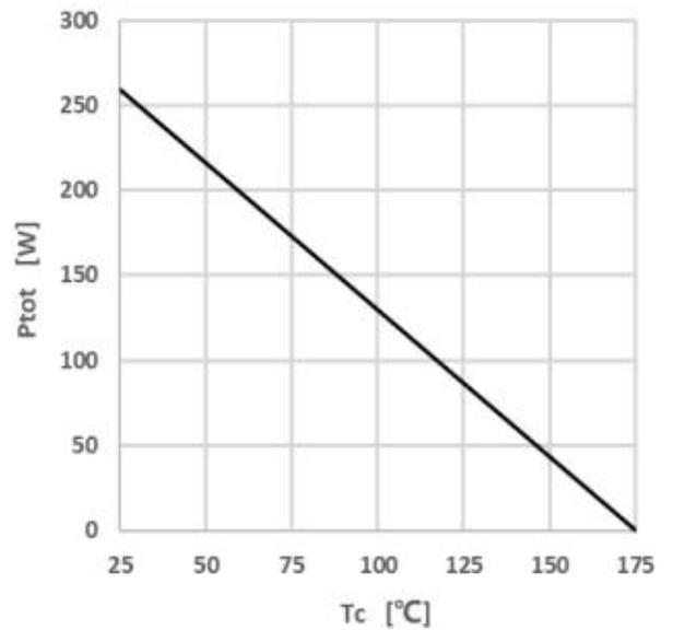
**Figure 4 Power Dissipation**
