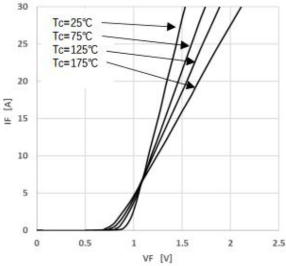
**Figure 1 Forward Characteristics**
