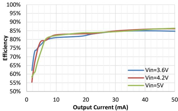
**Efficiency with 7LEDs**
