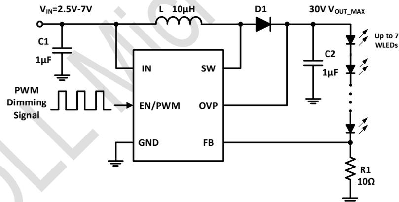
Figure 3. Dimming Control by a PWM Signal to EN Pin
