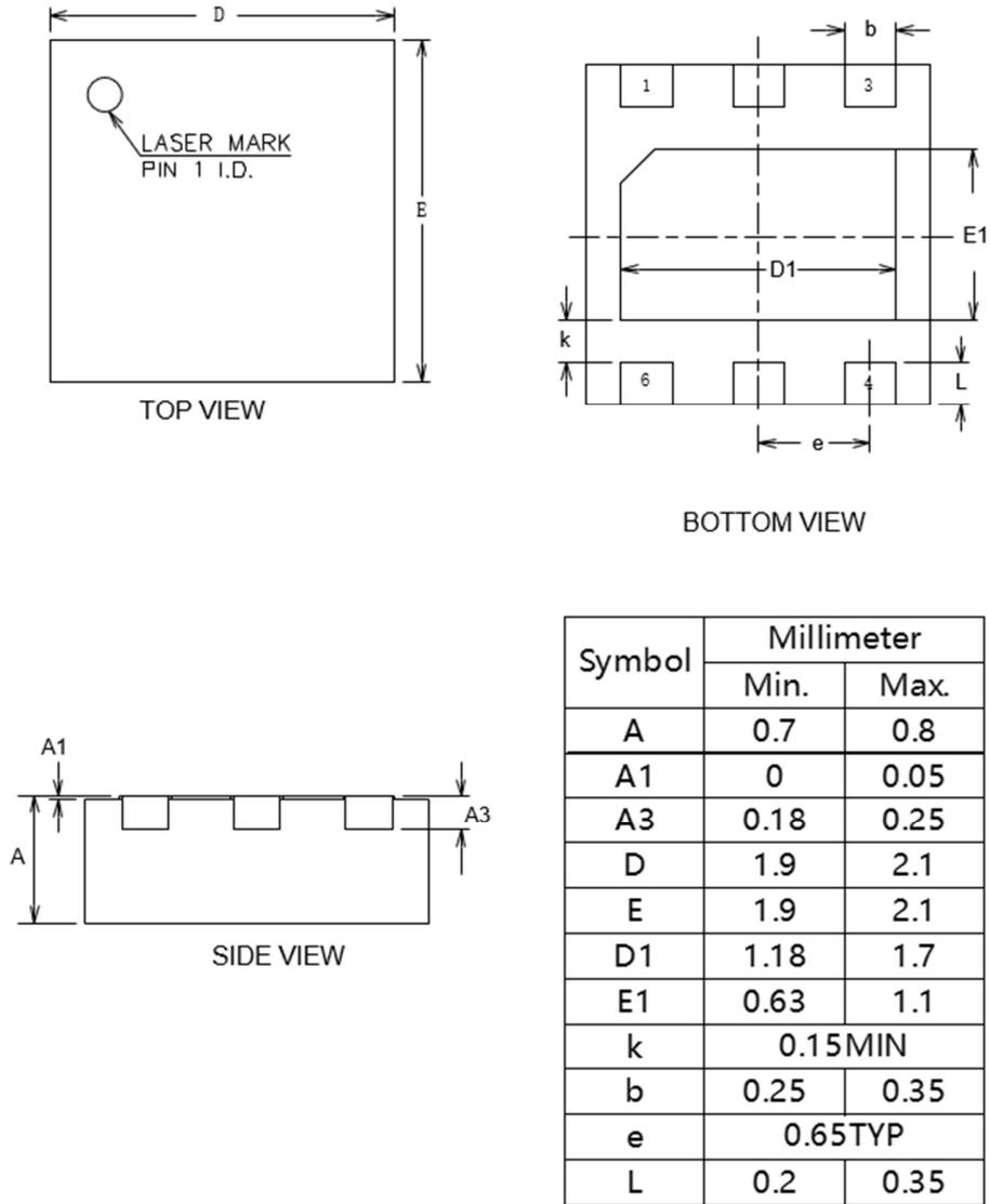
Figure 9. DFN2x2-6L Package, 2 mm x 2 mm Body
