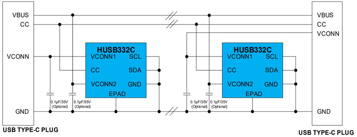
Figure 8. Two eMarkers Solution without VCONN Connected Through the Cable
