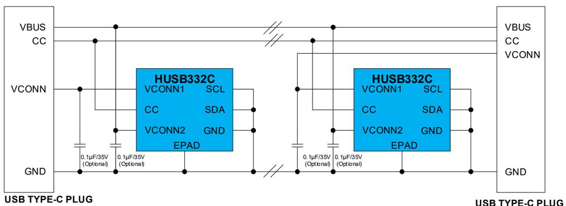
Figure 1. HUSB332C\_B44DA Typical Application Circuit
