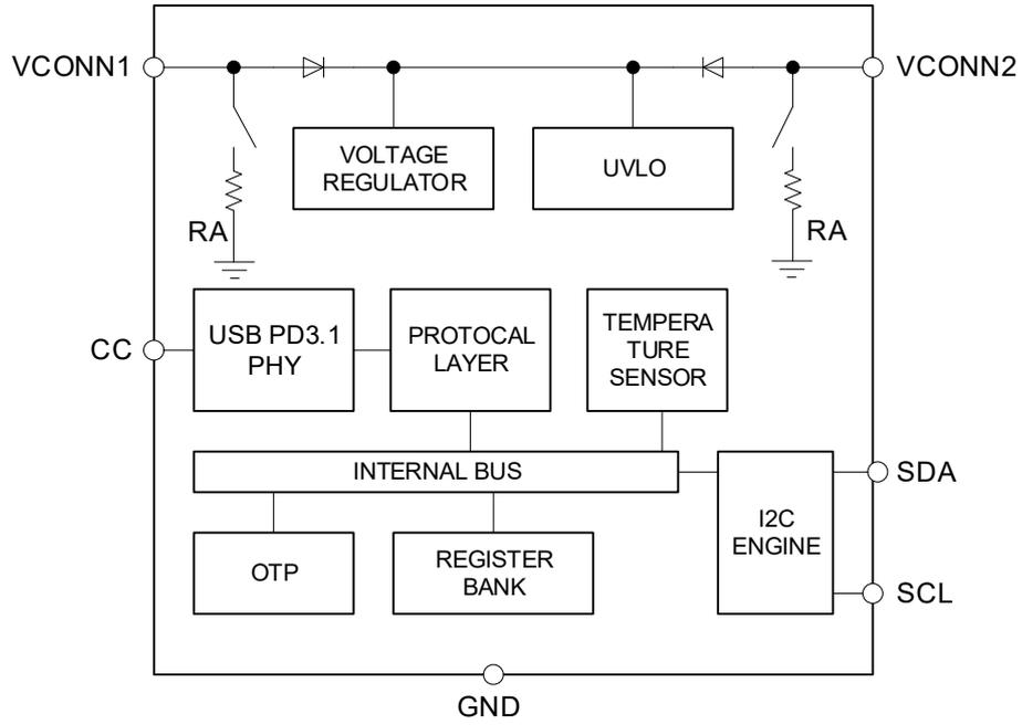
Figure 3. HUSB332C Functional Block Diagram
