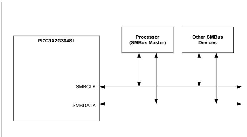
The SMBus interface on the PI7C9X2G304SL consists of one SMBus clock pin (SMBCLK), a SMBus data pin (SMBDATA), and 3 SMBus address pins (GPIO[5:7]). The SMBus clock pin provides or receives the clock signal. The SMBus data pin facilitates the data transmission and reception. Both of the clock and data pins are bi-directional. The SMBus address pins determine the address to which the PI7C9X2G304SL responds to. The SMBus address pins generate addresses according to the following table:
