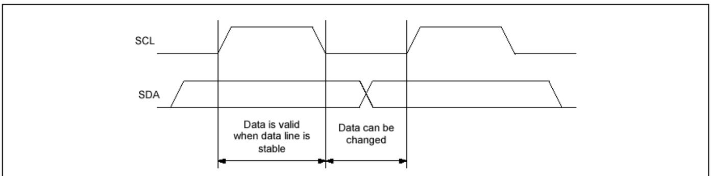
\*Note with caution that if the SDA data is changed while the SCL line is at high level, it will be treated as a START, RESTART, or STOP condition.
