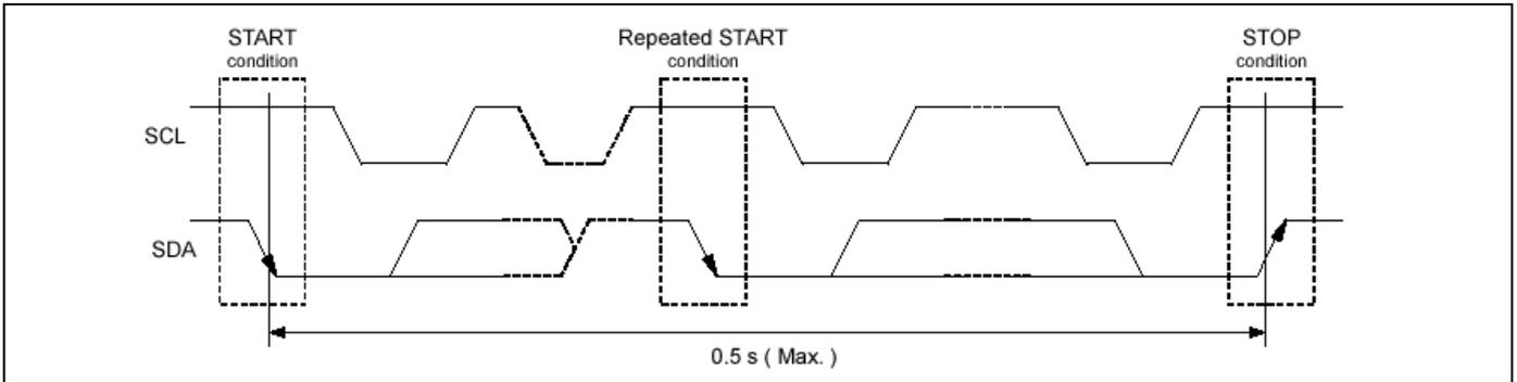
**Fig.2 Starting and stopping on I<sup>2</sup>C bus**
