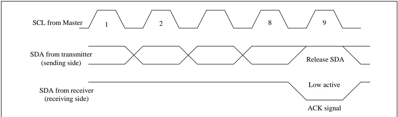
After transmitting the ACK signal, if the Master remains the receiver for transfer of the next byte, the SDA is released at the falling edge of the clock corresponding to the 9th bit of data on the SCL line. Data transfer resumes when the Master becomes the transmitter.
