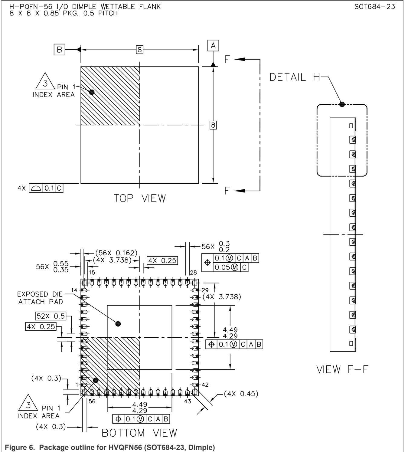
H-PQFN-56 I/O DIMPLE WETTABLE FLANK
