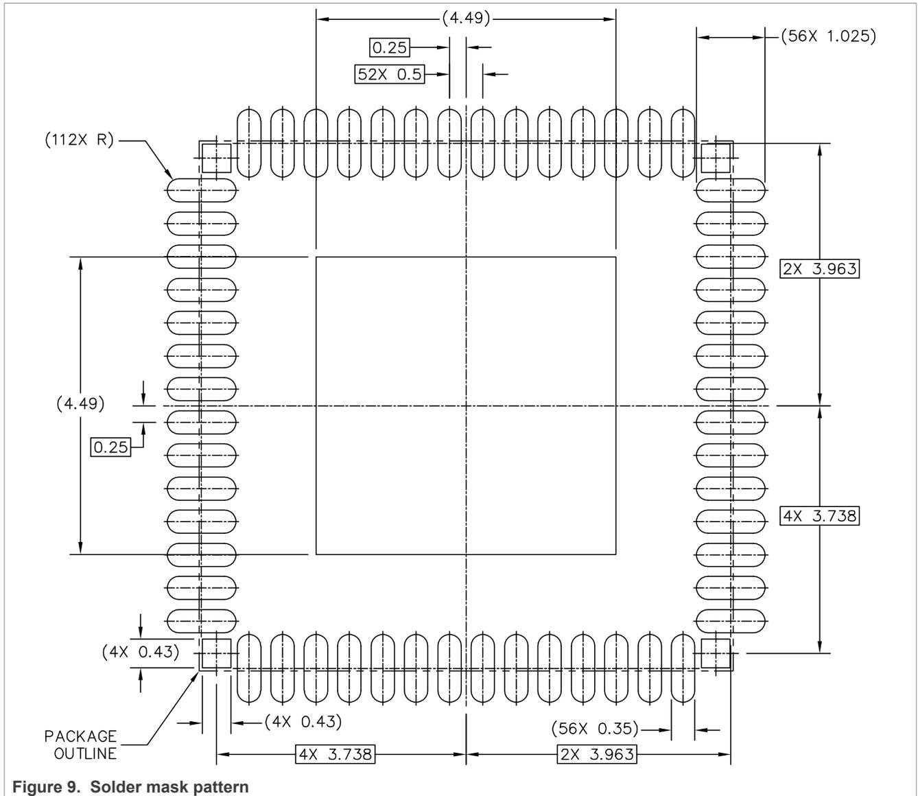
Figure 9. Solder mask pattern
