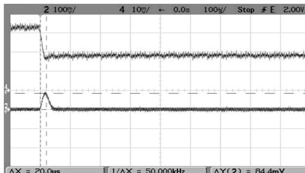
Step Load Transient Response ( $V_{in}=36V$ ,  $V_{out}=\text{nominal}$ ,  $\text{Clad}=0$ ,  $I_{out}=0.75A$  to  $1.5A$ ,  $\text{Slew}=1A/\mu\text{s}$ ,  $T_a=+25^\circ\text{C}$ .) Trace 2= $V_{out}$ , 100 mV/div. Trace 4= $I_{out}$ , 0.5A/div.
