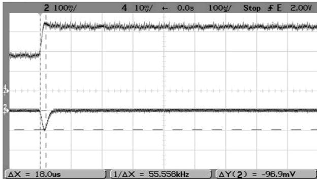
Step Load Transient Response ( $V_{in}=15V$ ,  $V_{out}=\text{nominal}$ ,  $\text{Cl}_{oad}=0$ ,  $I_{out}=1.0A$  to  $0.5A$ , Slew= $1A/\mu S$ ,  $T_a=+25^{\circ}C$ .) Trace 2= $V_{out}$ , 100 mV/div. Trace 4= $I_{out}$ , 0.5A/div.
