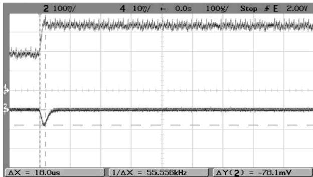
Step Load Transient Response ( $V_{in}=12V$ ,  $V_{out}=\text{nominal}$ ,  $\text{Clad}=0$ ,  $I_{out}=1.5A$  to  $0.75A$ ,  $\text{Slew}=1A/\mu S$ ,  $T_a=+25^\circ C$ .) Trace 2= $V_{out}$ , 100 mV/div. Trace 4= $I_{out}$ , 0.5A/div.
