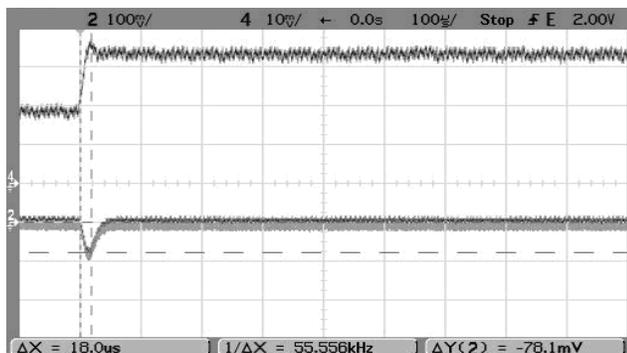
Step Load Transient Response ( $V_{in}=36V$ ,  $V_{out}=\text{nominal}$ ,  $\text{Clad}=0$ ,  $I_{out}=1.5A$  to  $0.75A$ ,  $\text{Slew}=1A/\mu\text{s}$ ,  $T_a=+25^\circ\text{C}$ .) Trace 2= $V_{out}$ , 100 mV/div. Trace 4= $I_{out}$ , 0.5A/div.
