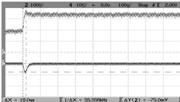
Step Load Transient Response ( $V_{in}=36V$ ,  $V_{out}=\text{nominal}$ ,  $\text{Clad}=0$ ,  $I_{out}=1.5A$  to  $0.75A$ ,  $\text{Slew}=1A/\mu S$ ,  $T_a=+25^\circ C$ .) Trace 2= $V_{out}$ , 100 mV/div. Trace 4= $I_{out}$ , 0.5A/div.
