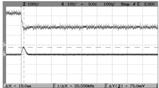
Step Load Transient Response ( $V_{in}=36V$ ,  $V_{out}=\text{nominal}$ ,  $\text{Clad}=0$ ,  $I_{out}=0.75A$  to  $1.5A$ ,  $\text{Slew}=1A/\mu S$ ,  $T_a=+25^\circ C$ .) Trace 2= $V_{out}$ , 100 mV/div. Trace 4= $I_{out}$ , 0.5A/div.
