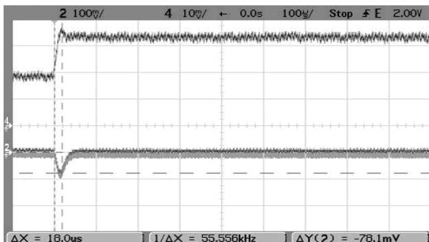
Step Load Transient Response ( $V_{in}=36V$ ,  $V_{out}=\text{nominal}$ ,  $\text{Cl}_{oad}=0$ ,  $I_{out}=1.0A$  to  $0.5A$ , Slew= $1A/\mu S$ ,  $T_a=+25^{\circ}C$ .) Trace 2= $V_{out}$ , 100 mV/div. Trace 4= $I_{out}$ , 0.5A/div.
