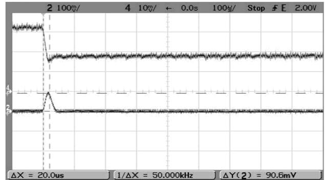
Step Load Transient Response ( $V_{in}=24V$ ,  $V_{out}=\text{nominal}$ ,  $\text{Cl}_{oad}=0$ ,  $I_{out}=0.5A$  to  $1.0A$ , Slew= $1A/\mu S$ ,  $T_a=+25^{\circ}C$ .) Trace 2= $V_{out}$ , 100 mV/div. Trace 4= $I_{out}$ , 0.5A/div.
