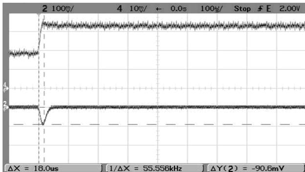
Step Load Transient Response ( $V_{in}=24V$ ,  $V_{out}=\text{nominal}$ ,  $\text{Cl}_{oad}=0$ ,  $I_{out}=1.0A$  to  $0.5A$ , Slew= $1A/\mu S$ ,  $T_a=+25^{\circ}C$ .) Trace 2= $V_{out}$ , 100 mV/div. Trace 4= $I_{out}$ , 0.5A/div.
