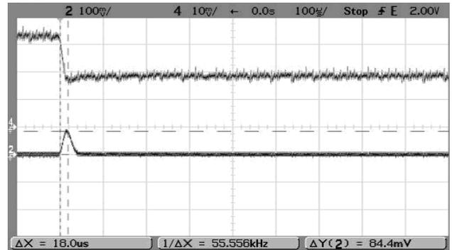
Step Load Transient Response ( $V_{in}=12V$ ,  $V_{out}=\text{nominal}$ ,  $\text{Clad}=0$ ,  $I_{out}=0.75A$  to  $1.5A$ ,  $\text{Slew}=1A/\mu S$ ,  $T_a=+25^\circ C$ .) Trace 2= $V_{out}$ , 100 mV/div. Trace 4= $I_{out}$ , 0.5A/div.
