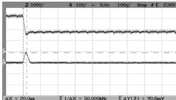
Step Load Transient Response ( $V_{in}=12V$ ,  $V_{out}=\text{nominal}$ ,  $\text{Clad}=0$ ,  $I_{out}=0.75A$  to  $1.5A$ ,  $\text{Slew}=1A/\mu\text{s}$ ,  $T_a=+25^\circ\text{C}$ .) Trace 2= $V_{out}$ , 100 mV/div. Trace 4= $I_{out}$ , 0.5A/div.
