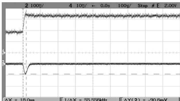
Step Load Transient Response ( $V_{in}=12V$ ,  $V_{out}=\text{nominal}$ ,  $\text{Clad}=0$ ,  $I_{out}=1.5A$  to  $0.75A$ ,  $\text{Slew}=1A/\mu\text{s}$ ,  $T_a=+25^\circ\text{C}$ .) Trace 2= $V_{out}$ , 100 mV/div. Trace 4= $I_{out}$ , 0.5A/div.
