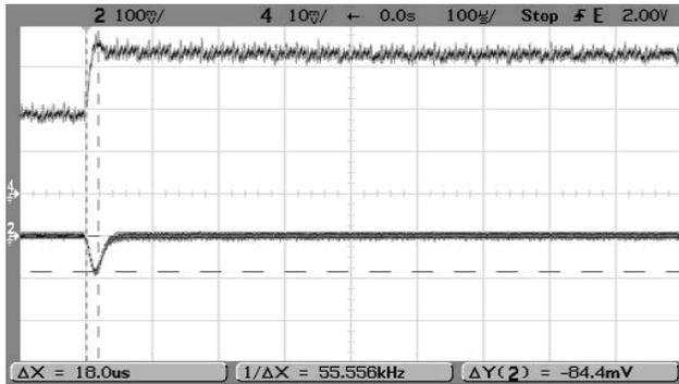
Step Load Transient Response ( $V_{in}=7V$ ,  $V_{out}=\text{nominal}$ ,  $\text{Clad}=0$ ,  $I_{out}=1.5A$  to  $0.75A$ ,  $\text{Slew}=1A/\mu S$ ,  $T_a=+25^\circ C$ .) Trace 2= $V_{out}$ , 100 mV/div. Trace 4= $I_{out}$ , 0.5A/div.
