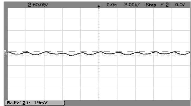
Output Ripple and Noise (Vin=36V, Vout=nominal, Iout=1A, Cload=0, Ta=+25°C, ScopeBW=100MHz)
