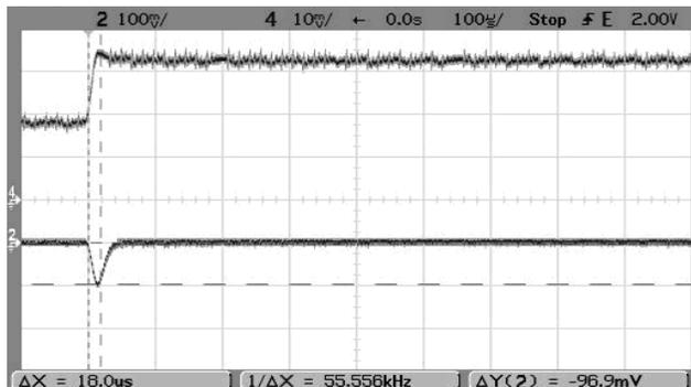
Step Load Transient Response ( $V_{in}=7V$ ,  $V_{out}=\text{nominal}$ ,  $\text{Clad}=0$ ,  $I_{out}=1.5A$  to  $0.75A$ ,  $\text{Slew}=1A/\mu\text{s}$ ,  $T_a=+25^\circ\text{C}$ .) Trace 2= $V_{out}$ , 100 mV/div. Trace 4= $I_{out}$ , 0.5A/div.
