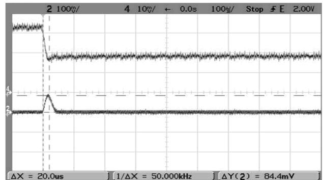
Step Load Transient Response ( $V_{in}=36V$ ,  $V_{out}=\text{nominal}$ ,  $\text{Cl}_{oad}=0$ ,  $I_{out}=0.5A$  to  $1.0A$ , Slew= $1A/\mu S$ ,  $T_a=+25^{\circ}C$ .) Trace 2= $V_{out}$ , 100 mV/div. Trace 4= $I_{out}$ , 0.5A/div.
