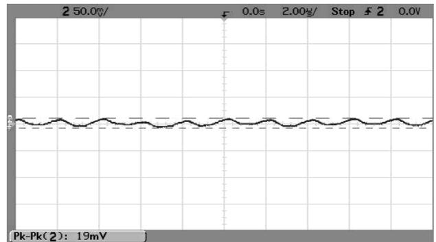
Output Ripple and Noise (Vin=36V, Vout=nominal, Iout=1.5A, Cload=0, Ta=+25°C., ScopeBW=100MHz)
